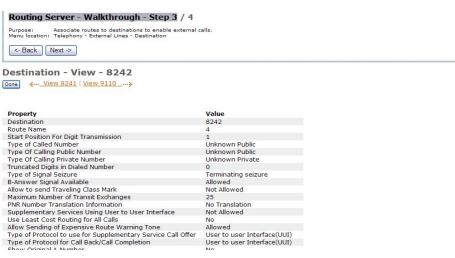
The screenshot below captures the full configuration for the SIP trunk to Destination 8242, the SR140 fax server, used in the sample configuration:
