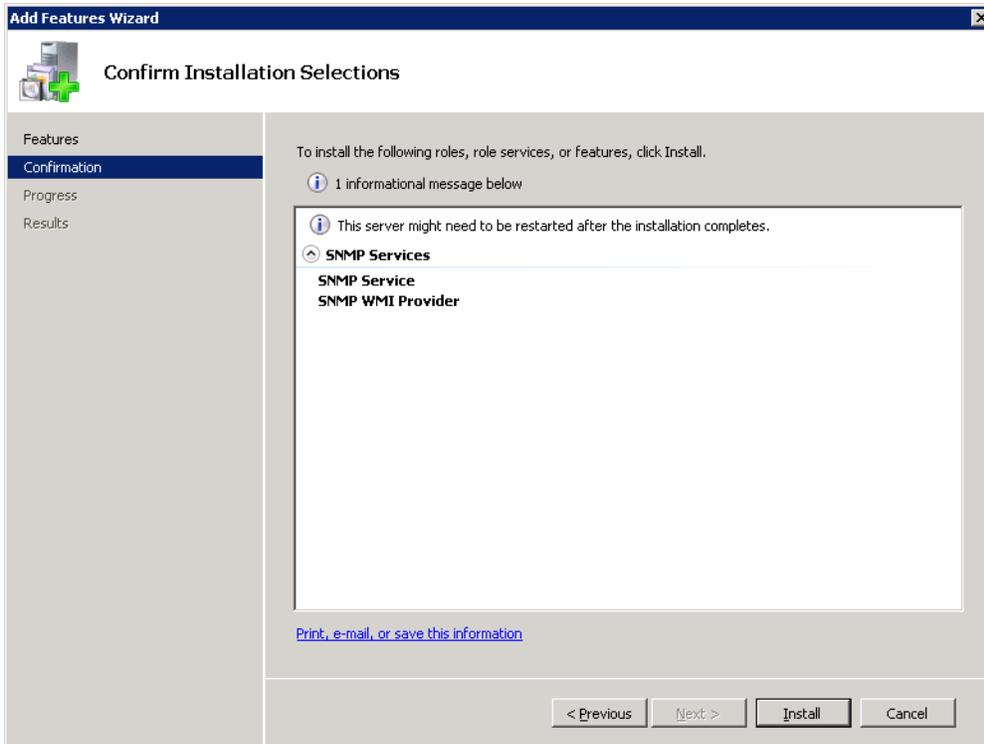
5. After the installation of the SNMP Services has finished, close the **Add Features Wizard** window. You will see the SNMP Services added to the list of installed features in the **Server Manager** window.
