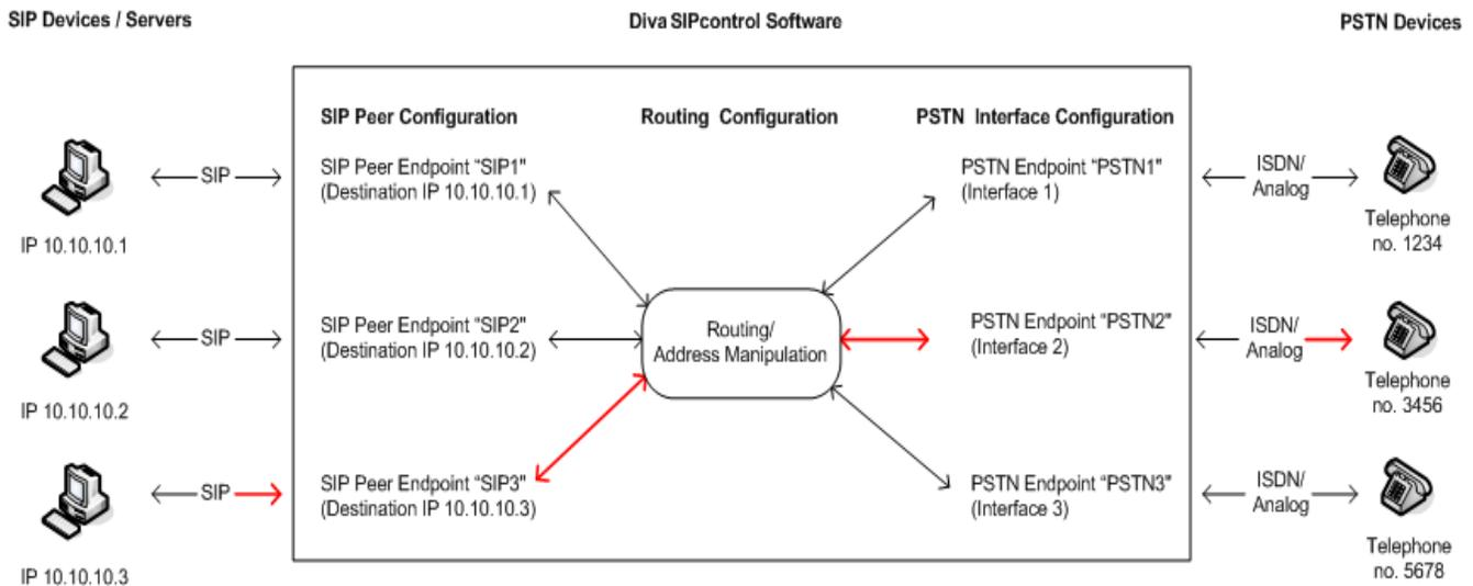
This graphic shows that an endpoint is only a virtual object of a real device. The endpoint saves the settings for the corresponding device. For example, if a call should be routed from SIP device 3 to PSTN device 2 as marked red in the graphic, then:
