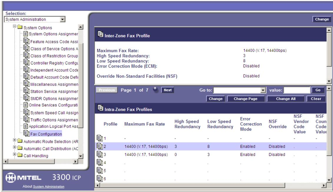
The Inter-Zone Fax Profile defines the FAX settings between the different zones in the network. There is only one Inter-Zone Fax Profile and it applies to all inter-zone fax communication. It defaults to V.29, 7200bps.
